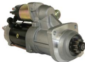
SDR0359 FOR 38MT SERIES, PLGR; 24-VOLT; CW; 10-TOOTH LESTER 6832; PIC 141-475; Used on Cummins ISB Engines REPL.: DELCO 8200024, 8200078, 8300023, 19026032
