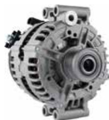
AB00394 For BMW IR/IF: 12-Volt; 180 Amp; Lester 11302; PIC 220-5484;
