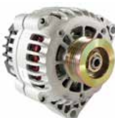
ADRO240-220 For CS130D Series IR/IF: 12-Volt; 220 Amp;
