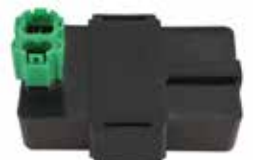
IKY6006 CDI Module For Kymco ATV, Scooters Capacitive Discharge Ignition
